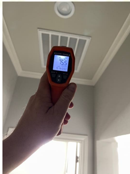
Temperature measured at a return for a split of near 20 degrees
