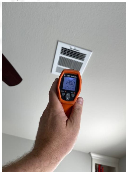
Temperature measured at a register while operating the furnace
