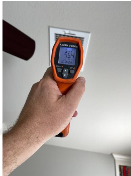
Temperature measured at a register while operating the AC
